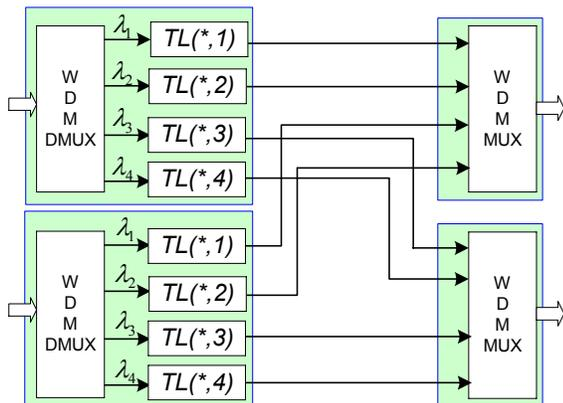
Fig. 3. Illustration of a  $2 \times 2$  FC-FλS switch (tunable lasers are coordinated by UTC signal, which is not shown in the figure).
