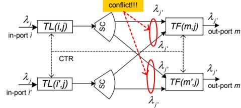
Fig. 6. One tunable filter replacing  $N$  ON/OFF switching elements.
