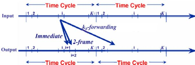
Fig. 2. Illustration of IF and NIF in time domain.
