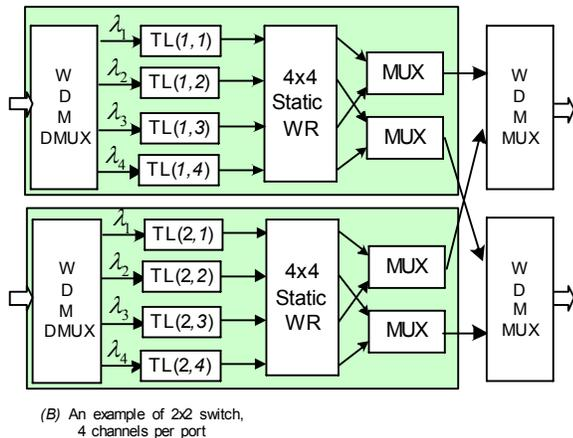
Fig. 4. (A) A design of WR-FλS, (B) a 2x2 switch (UTC signal is not shown).
