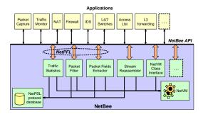
Figure 7 NetBee packet processing framework.
